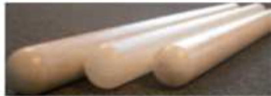
A) PCM E8 ENCAPSULATED IN HDPE TUBES B) PCM TANK DESIGN FIGURE 12 THE PCM E10 ENCAPSULATED IN HDPE TUBES AND PCM TANK DESIGN
