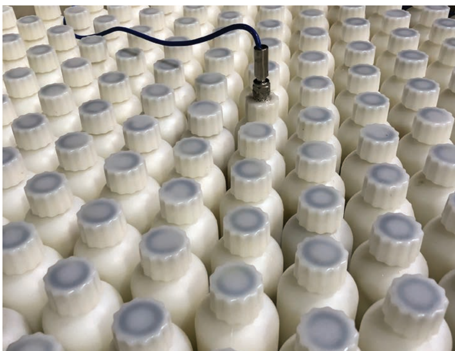
Figure 2.37 - Close-up of PCM Tubes
